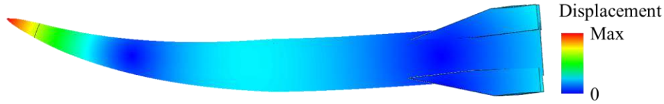
Figure 4: First lateral and longitudinal bending modes
