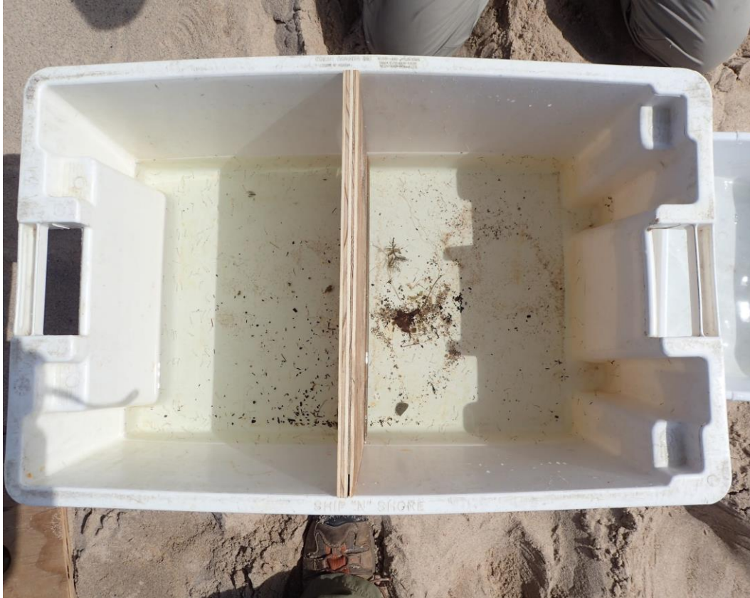
Figure 18: Light-box used to separate coregonid larvae into cisco and lake whitefish. This light-box with larvae inside was left covered for 30 minutes for larvae to sort themselves along a light gradient. After the allotted time, the wooden partition was placed in the middle of the light-box (shown). Larvae on the light side of the box were processed for gut contents. Photo by Jillian Mayer.
