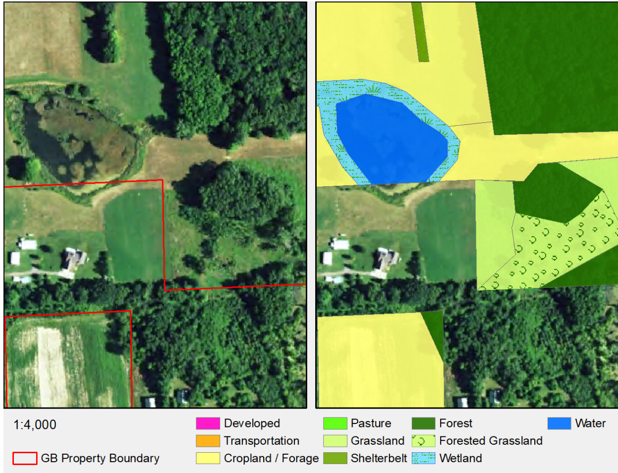
Figure 3.2: Example of NAIP imagery with Greenbelt parcel boundaries and classification polygons overlaid.
