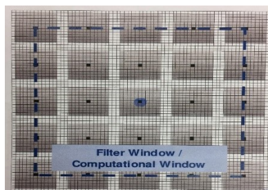
Figure 2: Filter window for strain calculation
