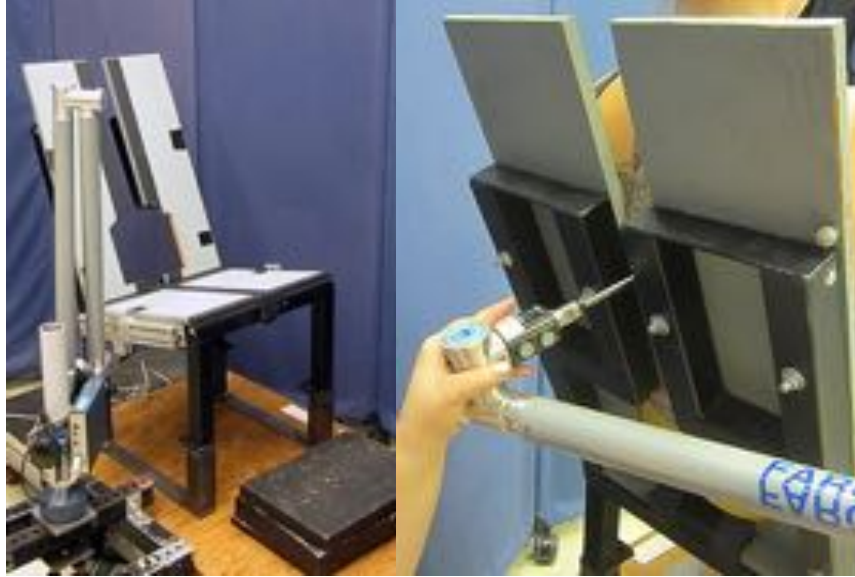
Figure 9. Hardseat with back opening (left) that allows access to posterior spine and pelvis as shown in center photo. Example of head IMU location being digitized with FARO Arm (right)
