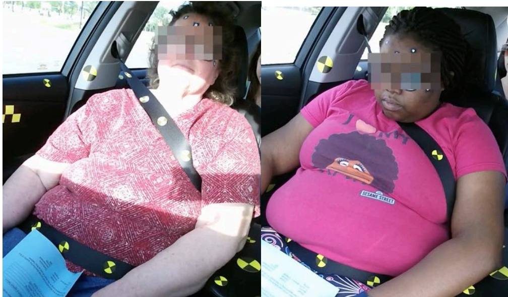
Figure 54. High belt routing on the torsos of two women with high BMI.
