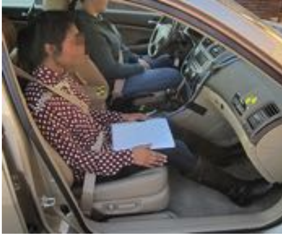
Figure 21. Testing posture: feet slid forward on heels and hands on thighs; questionnaire taped to thighs to prevent participant lifting it and blocking Kinect camera.
