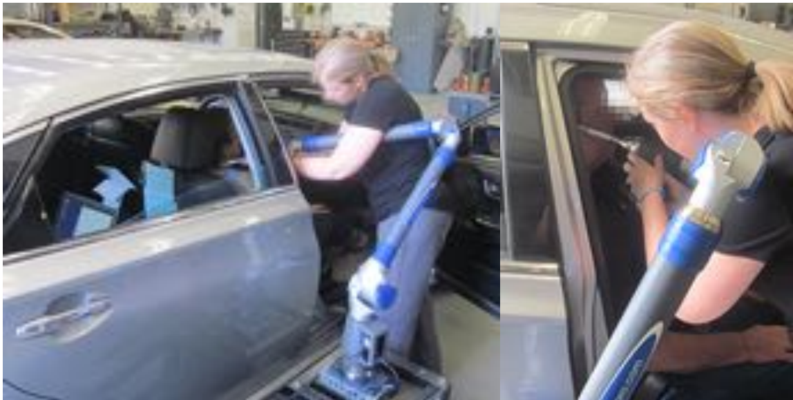
Figure 20. Investigator using FARO Arm to digitize points on participant, vehicle, and belt
