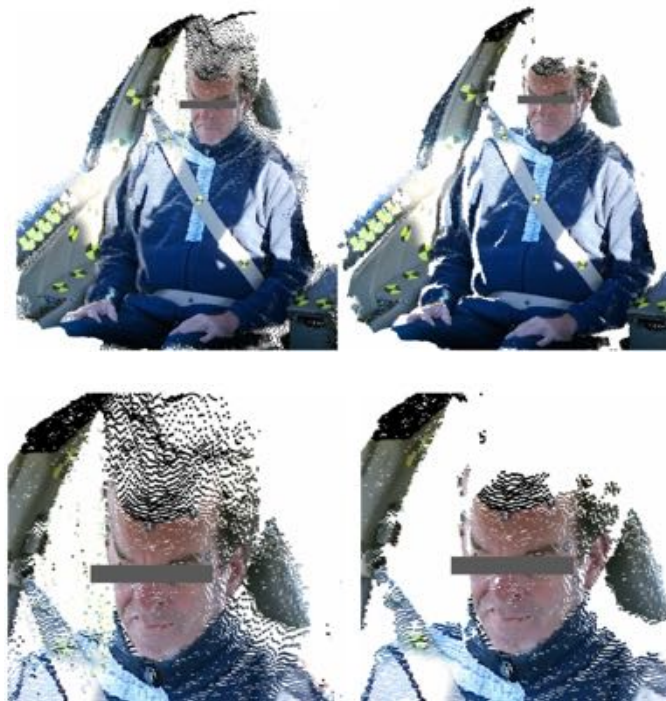
Figure 24. Processed Kinect depth data with RGB. Before (left) and after (right) flying pixel artifact filtering.
