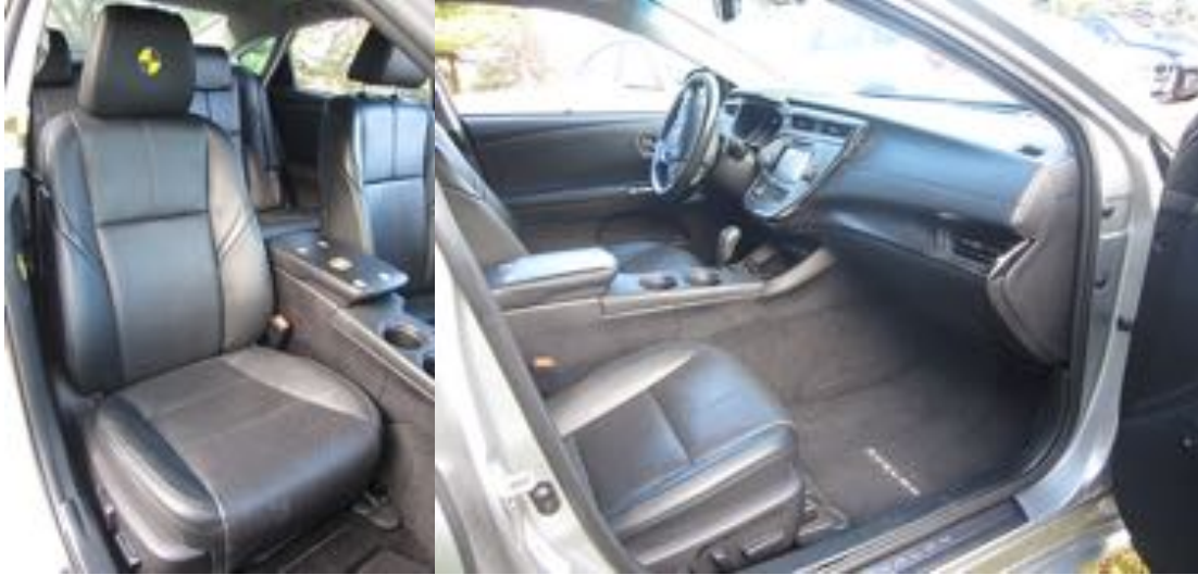
Figure 2. Front passenger seating area with seat set to the lowest position, flattest cushion angle, and a back angle of 23 degrees (SAE J826) and moved fully rearward on seat track.
