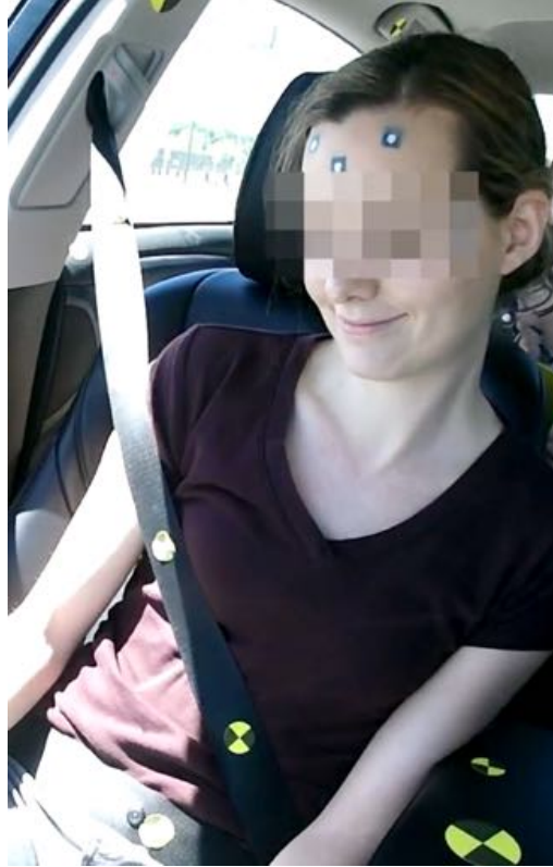
Figure 55. Belt off the shoulder of a participant during the turn-and-brake event. Note the elbow between the torso and console.
