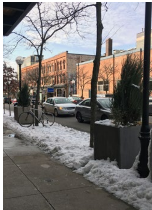
Figure 5: Planters along the frontage of Starbucks stand too high for sitting and have narrow ledges.
