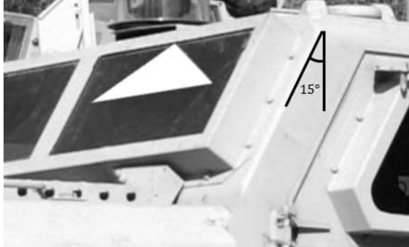
Figure 2.2: The placement of the monopole antenna in the windshield with a 15^\circ tilt. The ground plane is fabricated on the inside of the window glass and is electrically attached to the metallic body of the vehicle.
