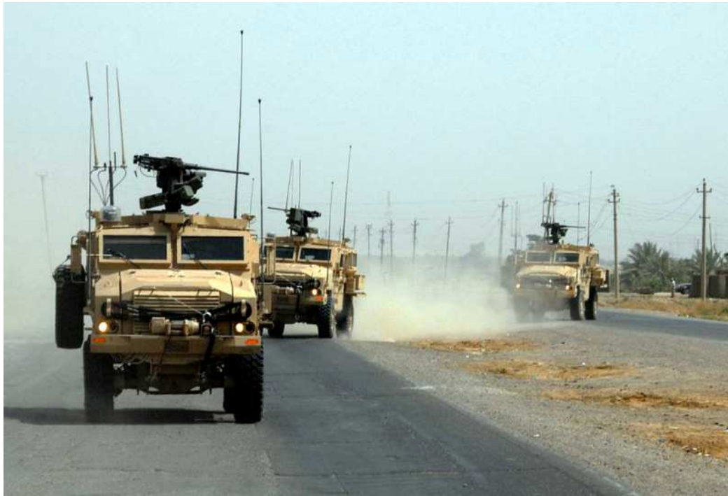
Figure 1.3: Military vehicles carry multiple vertical monopole or dipole antennas for ground communication purposes. Such antennas create air drag and increase visibility.
