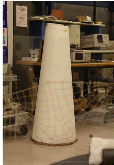
Figure 2.51: Fabricated meshed monopole antenna and meshed ground plane using conductive paint silk printing.
