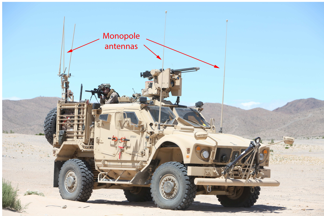
Figure 2.16: The transparent antennas replace the commonly used monopole antennas and improve their performance. The windshield and side windows of MATV are good candidates for antenna placement.
