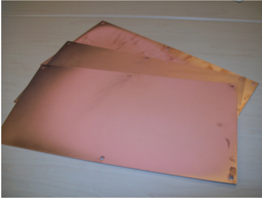
Figure 2.48: polycarbonate sheets metalized using electro-less plating
