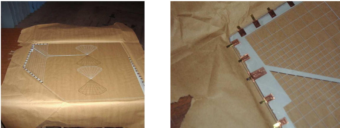
Figure 2.71: grounding points attached to the edges of the antenna layer to ensure an electric connection between the metallic covers and the window frame.
