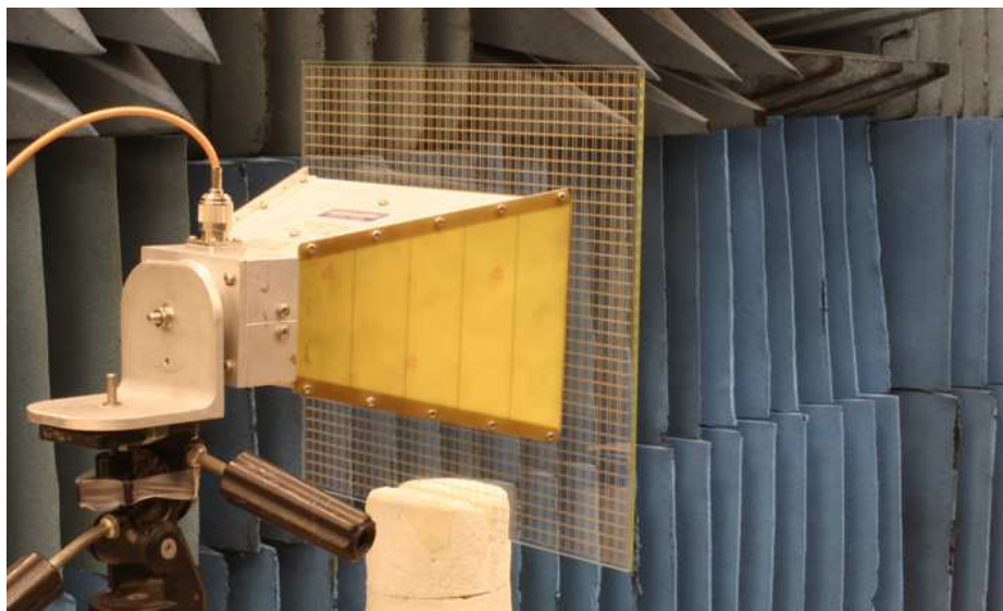
Figure 3.23: Measurement Setup. The transmitting antenna is placed far enough for the plane wave approximation to be fairly accurate.
