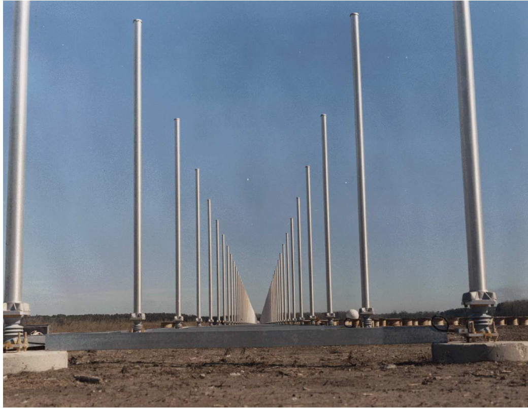
Figure 1.2: An over-the-horizon radar consisting of a long array of monopole antennas. Photo courtesy of the US Navy, https://commons.wikimedia.org/w/index.php?curid=9766600
