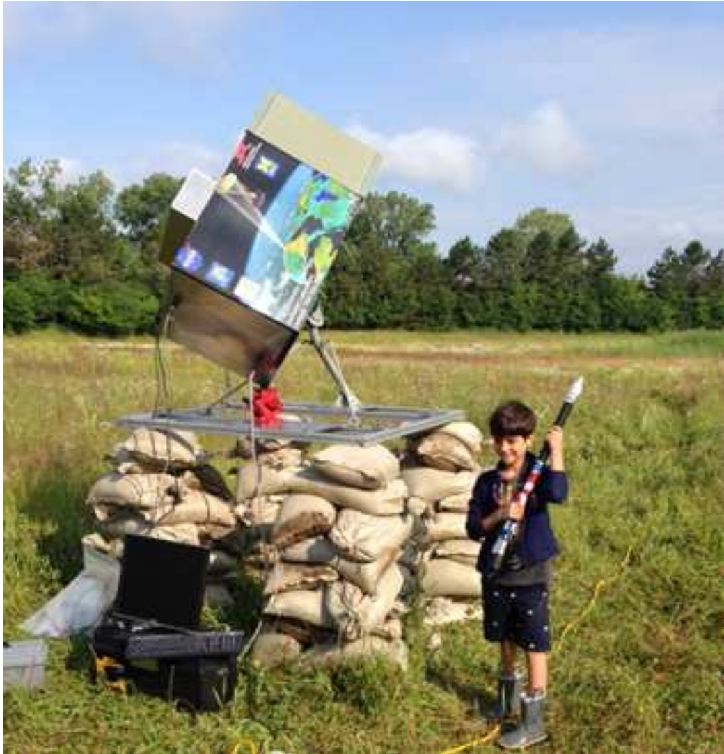
Figure 5.8: Measurement setup in the initial test location. The PARC is elevated to prevent ground reflections through the PARC's antenna sidelobe from increasing the coupling between the OMT ports. The PARC is controlled manually during the initial test period using an external monitor and keyboard. This procedure is performed autonomously after the final deployment of the PARC.
