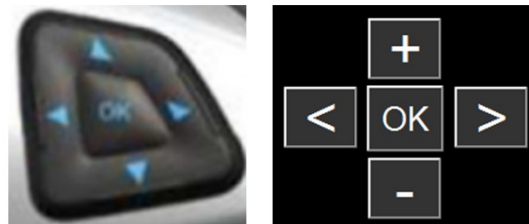
Figure 8.4 – Five-way-button device (on the left) and its digital mockup (on the right)
