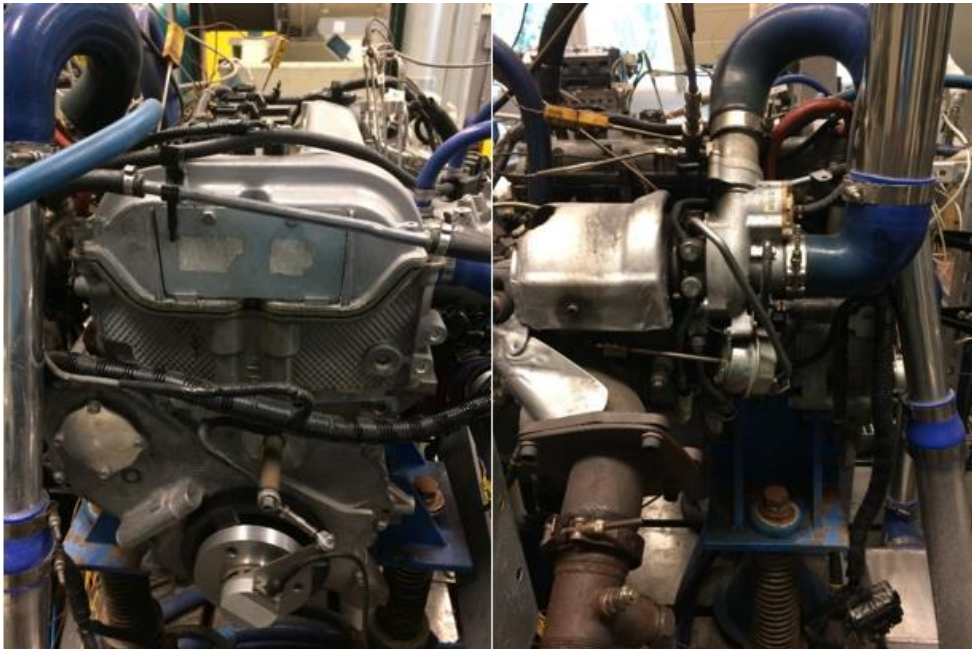
Figure 7. Images of the LNF Engine used for Soot Collection
