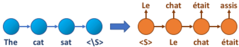
Figure 1.2: An example seq2seq model for machine translation. Blue circles are cells of the encoder and orange are cells of the decoder.
