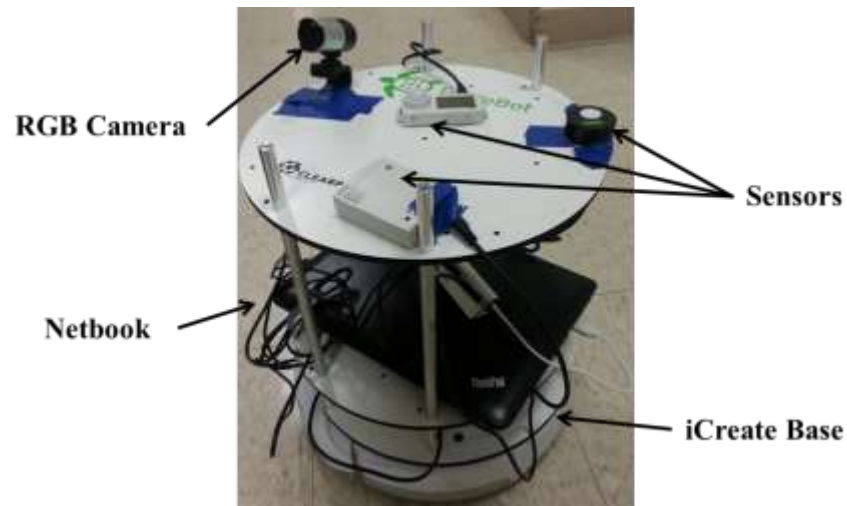
Figure 3.1 Components of mobile robot used for ambient data collection in buildings
