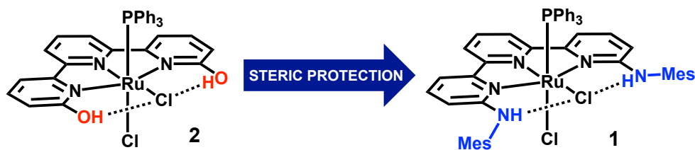
Figure 2-3: Catalyst 1 features steric protection in the form of 2,4,6-trimethylphenyl (Mes) groups compared to catalyst 2 .
