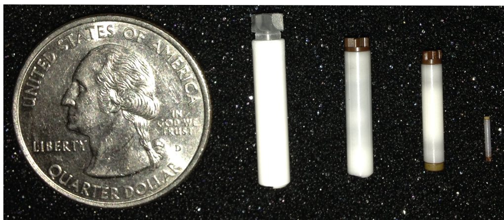
FIGURE 1.4: Bruker MAS rotors. The diameters from left to right are: 4 mm, 3.2 mm, 2.5 mm, and 0.7mm. Maximum spinning speeds increase with decreasing rotor sizes. 4 mm rotors typically max around 15 kHz while the 0.7 mm rotor has an upper limit of 111 kHz set by the manufacture. The quarter is included for reference.
