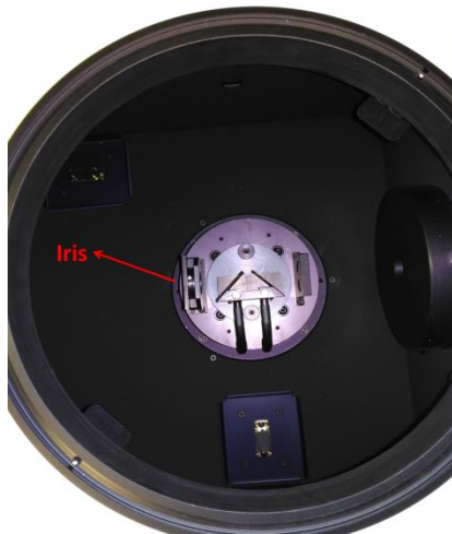
Figure 6.12. Sample compartment with iris
