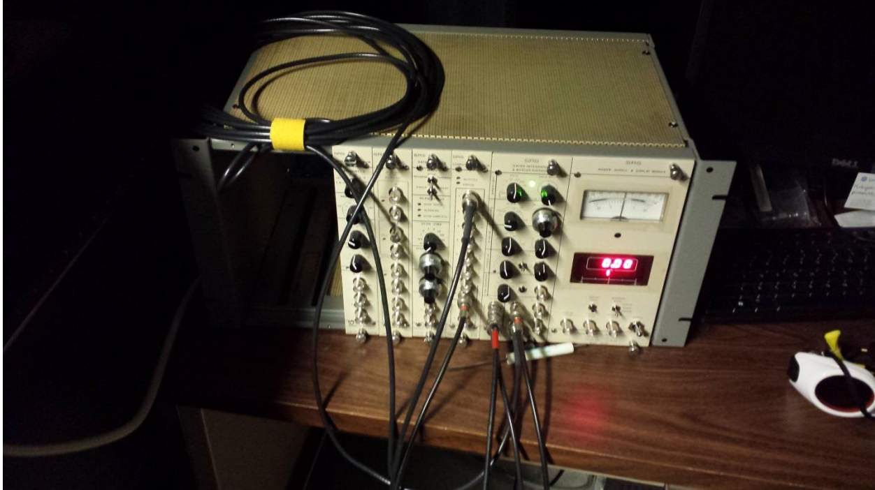
Figure 5.2.9. SRS 250 gated integrator
