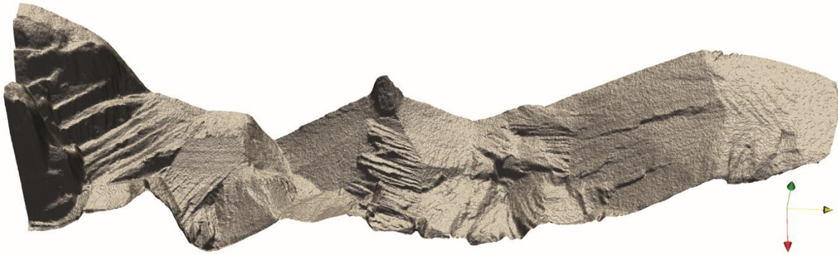
Figure C. 1 - Fracture surface from a WE43 magnesium foil specimen investigated using ultrasonic fatigue. a) Electron microscopy is used to characterize the fracture surface and to produce a b) 3-dimensional surface mesh of surface morphology using tilt photogrammetry in Alicona MeX.
