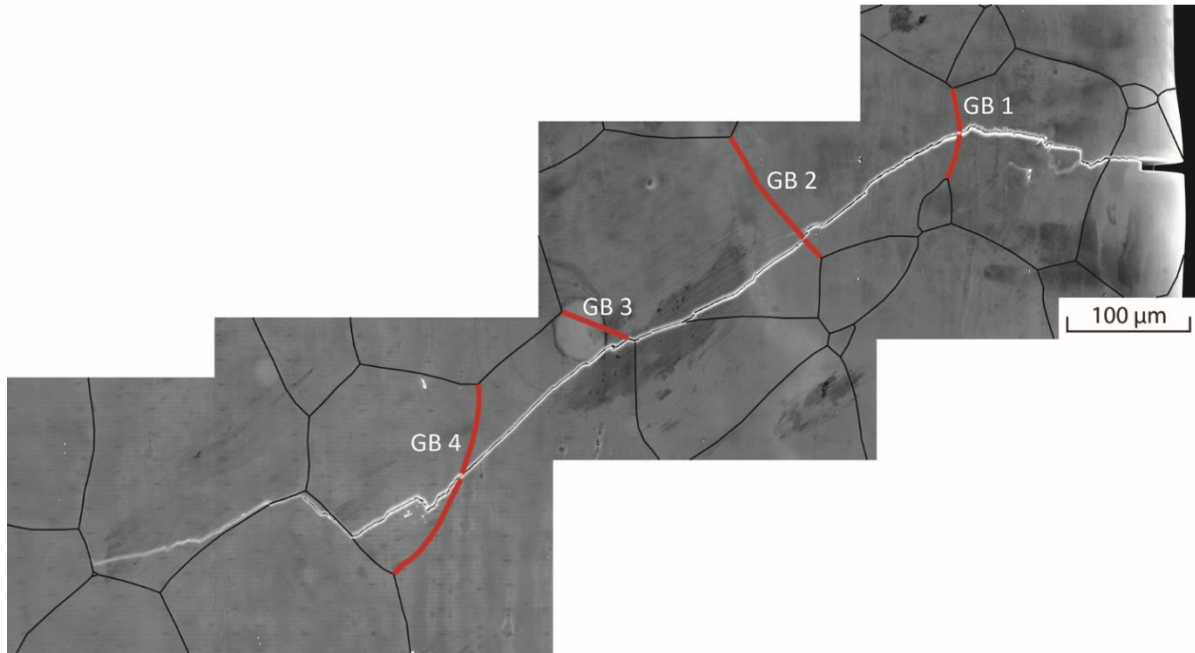
Figure 5.19 – Fatigue crack growth in foil specimen F4, exhibiting predominantly crystallographic transgranular growth along the basal slip system.
