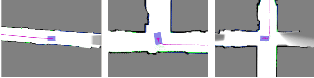
Figure 3.2: Example LPMs constructed during navigation of an office building.
