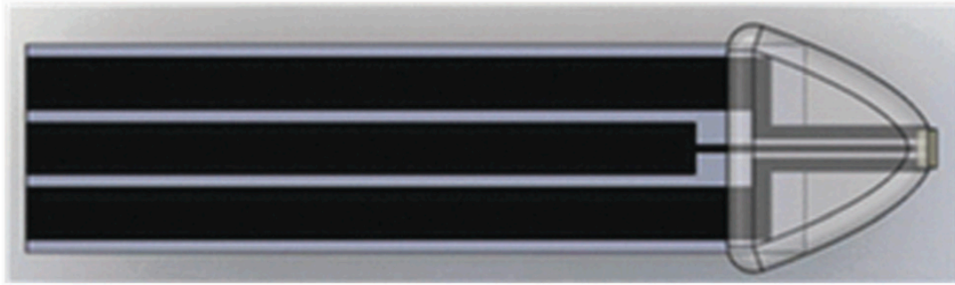
Figure 6.1. Potential design of tear glucose sensor featuring a soft housing for holding the absorptive material that may sit directly above the sensing area. 3
