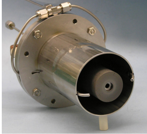
Figure 4.3: The JPL-designed high-current LaB 6 hollow cathode used during this work. The tubes at the 3 and 9 o'clock positions near the exit orifice of the cathode are the external gas injectors.
