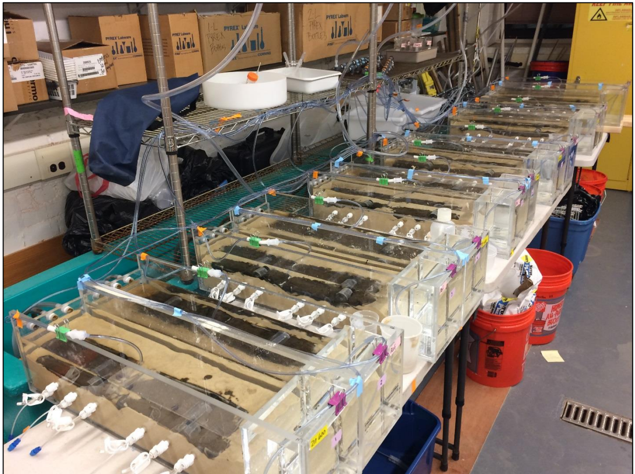
Figure 3.2. The 12-flume experiment was setup in the laboratory. The upstream end of the flume is on the right and downstream is on the left, and surface water flows from right to left. Rhizon sampling ports for temporal porewater sampling are located along the sides of each flume.
