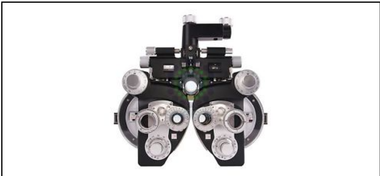
Figure 3.1. Phoropter. Optometrists use the phoropter to test several dimensions of vision individually and in conjunction with one another.
