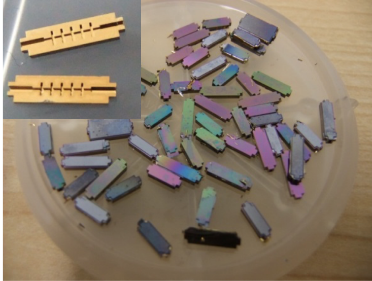
Figure 8.5: Fabricated SSPP components; in the left corner: halves of the SSPP components is shown to illustrate the grooves.
