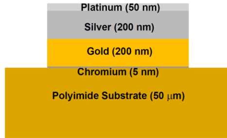
Figure 3-2. Metal stack design durable to process parameters.
