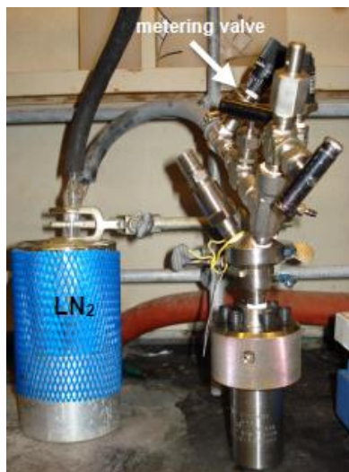
Figure 5.15. Picture of Reactor Being Worked-up when Recycling Ir@MIL
