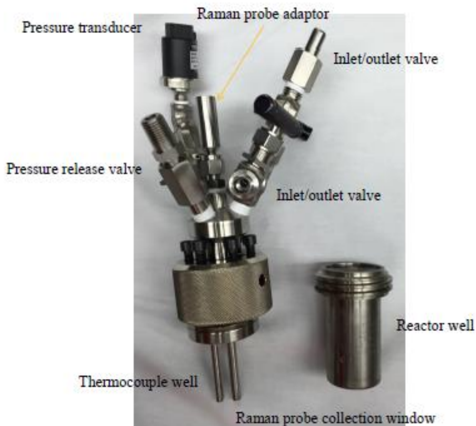
Figure 2.20. Picture of reactor type B with the parts of the reactor labeled.
