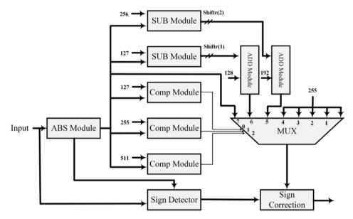
Fig. 6. Piecewise linear activation function module
