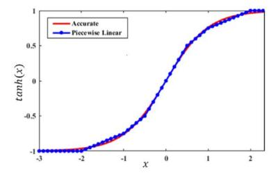
Fig. 4. Piecewise linearization of tanh(x)
