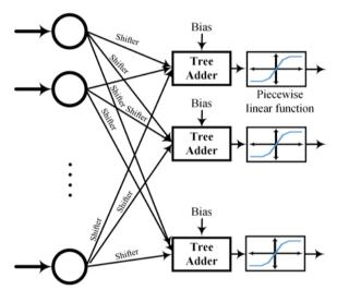
Fig. 5. Hardware structure of the simplified ANN
