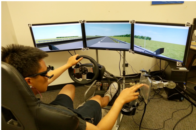
Figure 3: Driving simulator and secondary task setup. A volunteer is driving with the simulated vehicle while doing visual-search task on a touchscreen. Markers are placed on each monitor and the touchscreen to identify surfaces for eye-tracking.
