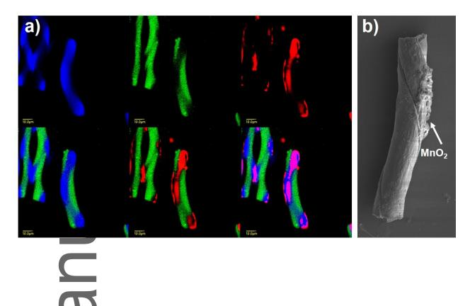
**Figure 5.** a) CLSM images of helical microcylinders decorated with a red dye in one compartment. b) SEM image of helical microcylinders decorated with MnO<sub>2</sub> nanoparticles on one compartment (the length of microcylinder is identical with that of microcylinder provided in Figure 5a).
