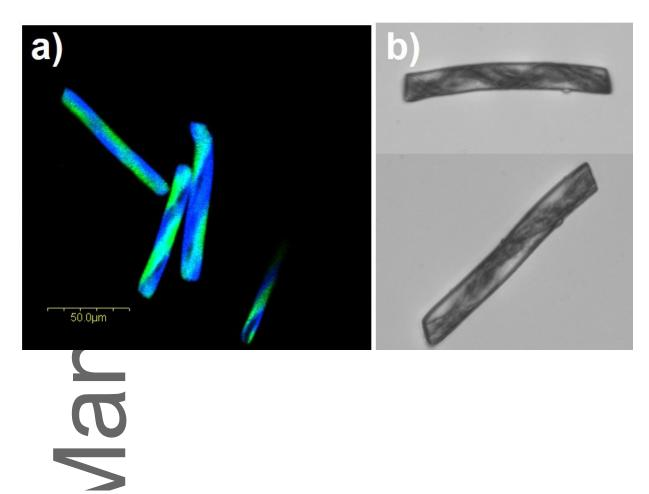
Figure 4. a) CLSM and b) optical microscopy images of microcylinders having inner helical architecture with magnetic nanoparticles in one compartment. The cylinders are sectioned at 70  $\mu$ m. Optical microscopy images show that the pitch size of the helical structure can be controlled.
