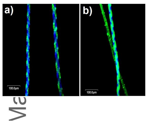
Figure 1. CLSM images of helically compartmentalized microfibers with (a) left and (b) right handedness (diameter:  $30 \mu m$ , pitch size:  $100 \mu m$ )
