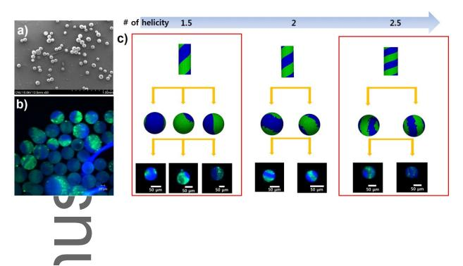
**Figure 6.** a) SEM image of microspheres prepared by shape evolution of helical microcylinders. b) CLSM image of helical microspheres. c) Schematic illustration of helical microcylinders with various pitch sizes (top row), and corresponding microspheres prepared by shape evolution (middle row, viewed from different angle), which is calculated by the Surface Evolver program. CLSM images of experimental data are also demonstrated according to their matched inner architecture (bottom row).
