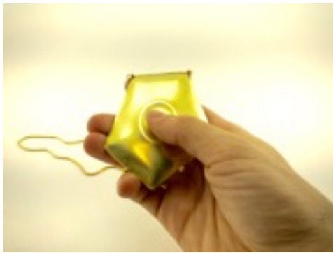
Made from brass, the shape was formed from laser cut acrylic dies on a hydraulic press.
