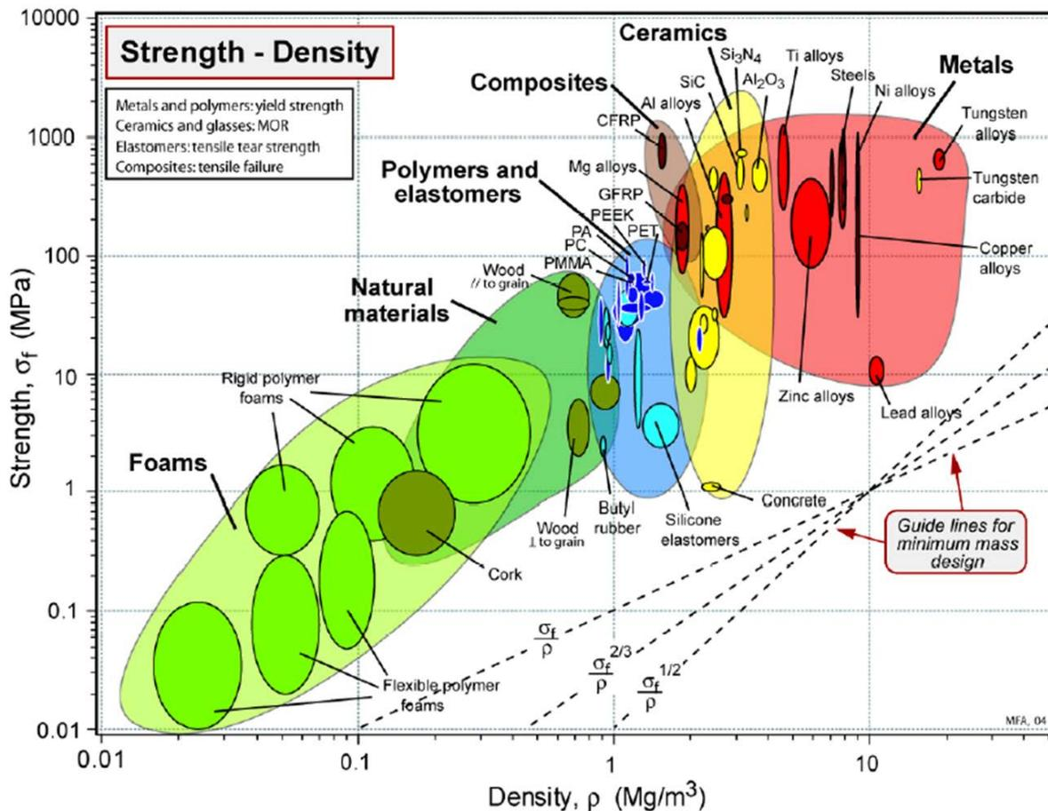
**Figure 5: Software tools allow for the rapid selection of candidate materials based on combination of multiple performance parameters. This figure illustrates how various materials rank based on strength and density.**
