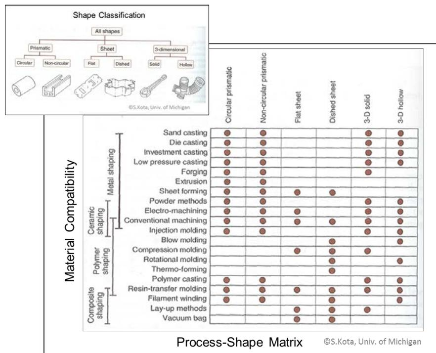
**Figure 6: Process Shape Matrix for Process Selection**
