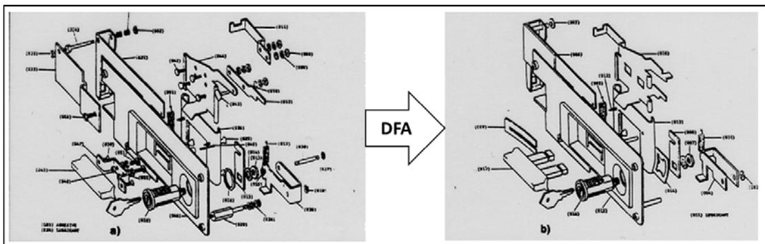
**Figure 7: Decrease in part count and complexity using the Design for Assembly principles**
