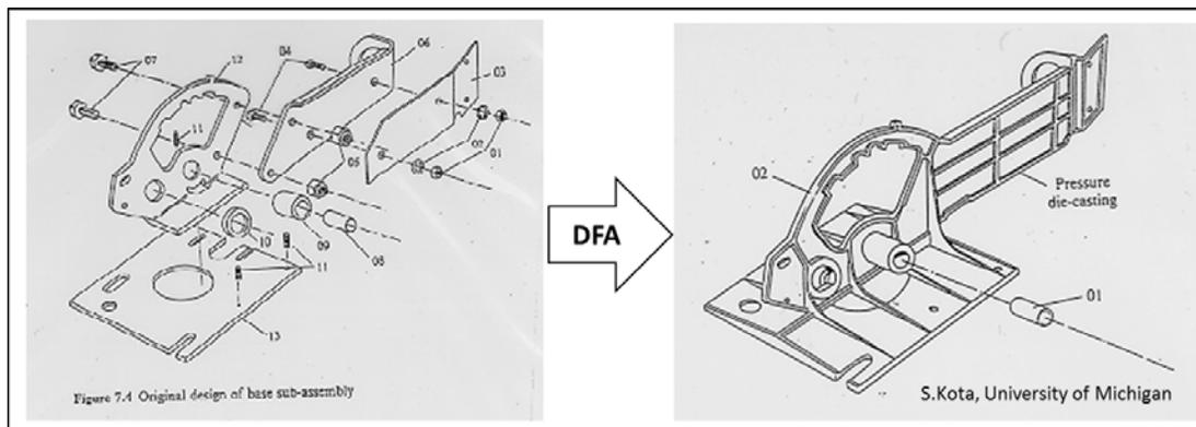
**Figure 8: Overall part count can be drastically decreased using Design for Assembly techniques. In this example, the overall part-count was reduced from 13 parts to 2 parts.**
