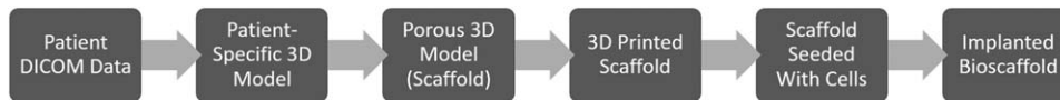
Fig. 6. Computer-aided design and 3D printing methodology for patient-specific cartilage tissue engineering. Digital Imaging and Communications in Medicine (DICOM) data of the anatomic structure of interest is acquired and used to generate a three-dimensional model of the structure. The model is then converted into a porous structure using negative Boolean operations and manufactured from polycaprolactone using a selective laser sintering 3D printer. The bioresorbable scaffold is then seeded with cells suspended in a hyaluronic acid/collagen hydrogel prior to implantation. (Adapted from Otolaryngology-Head & Neck Surgery , Volume 152, Issue 1, DA Zopf, AG Mitsak, CL Flanagan, et al. Computer-aided-designed, 3-dimensionally printed porous tissue bioscaffolds for craniofacial soft tissue reconstruction, 57–62, Copyright (2015), with permission from SAGE Publishing). 3D = three-dimensional.
