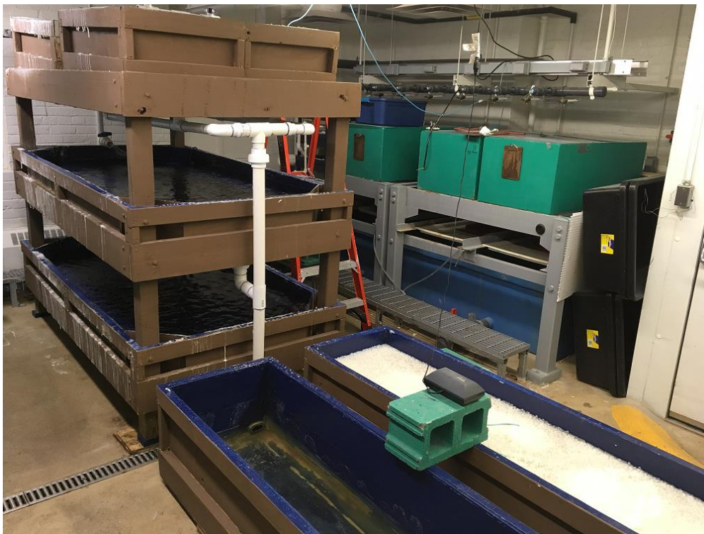
Figure 1. Pilot-scale RAS with four small rearing tanks and two large rearing tanks in stacked configuration. Through recirculation, all rearing tanks directly discharge water into aerated biofilter containing Kaldnes K1 media and directly receive water from sump tank.
