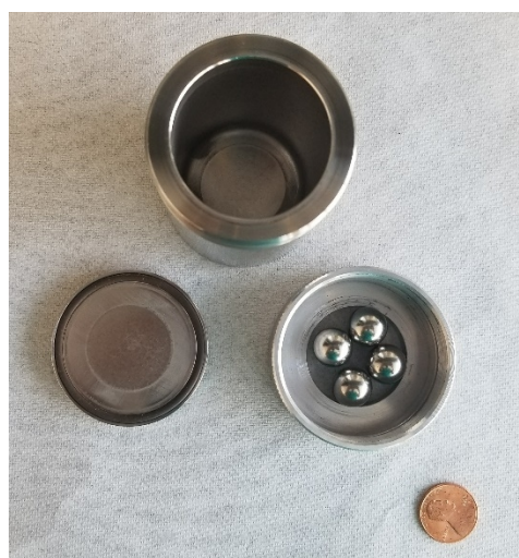
Figure 22. a) SPEX 8007 Stainless Steel vial b) Open vial with all components and stainless-steel balls placed next to a cent coin for reference
