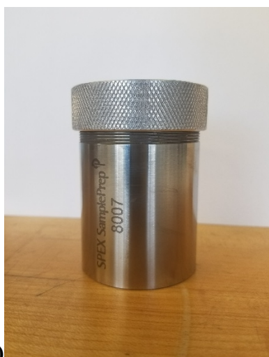
Figure 22. a) SPEX 8007 Stainless Steel vial b) Open vial with all components and stainless-steel balls placed next to a cent coin for reference
