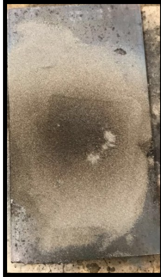
Figure 5.11: Heated substrate with 2 layers of SS 41C powder 1mm each
