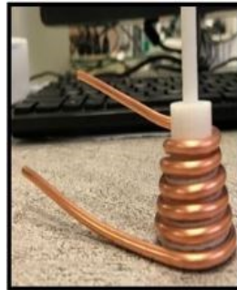
Figure 5.8: Copper tubing wound around a 3D printed fixture
