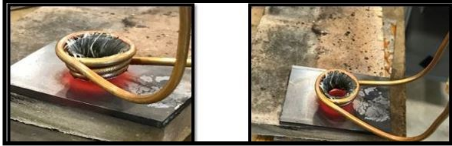
Figure 5.9: Images of heating trials with a 4 turn conical coil with Alphaform MF applied on the inner side of the coil
