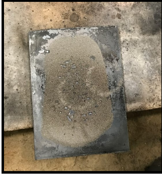
Figure 5.10: Substrate with SS 41C powder after heating trial
