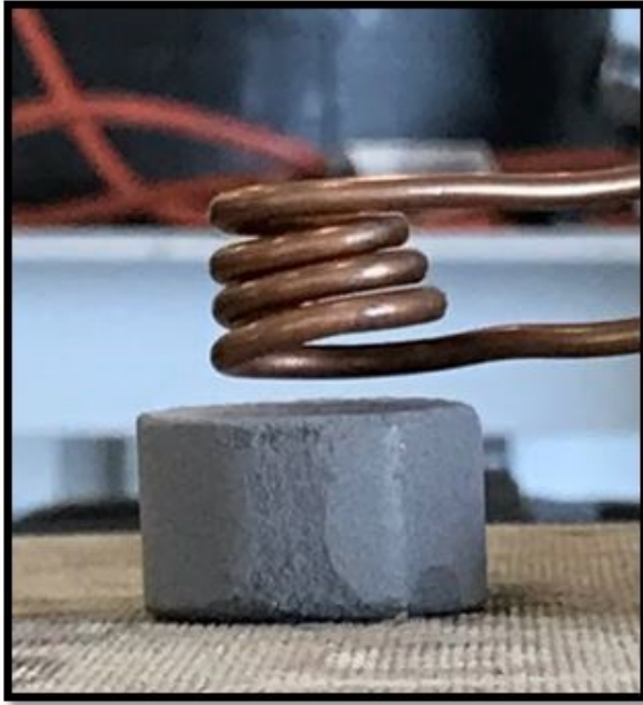
Figure 5.3: SS 41C powder compact tested out with a 4 turn induction coil (left) and the SS 41C powder compact being made on the molding press (right)
