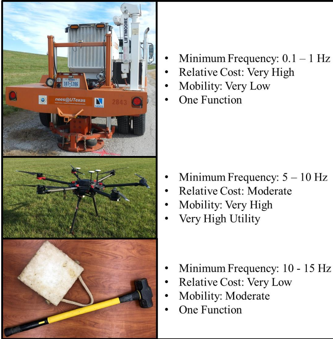
Figure 5-8: Fundamental comparison of seismic surface wave sources
