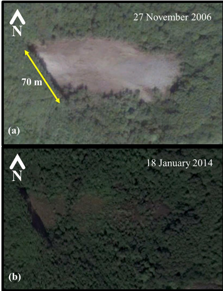
Figure 3-16: Satellite images of Small Awini Landslide (a) about 1 month after the 2006 Kiholo Bay earthquake and (b) in January 2014
