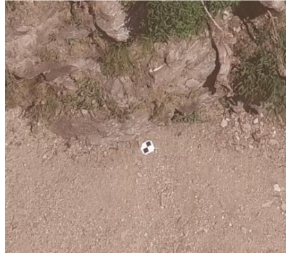
Figure 3-5: Example of GCP visible in a UAV-collected image
