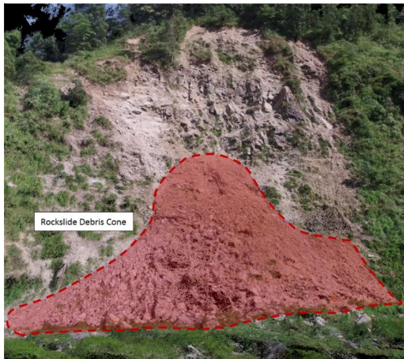
Figure 3-13: Point cloud overview of landslide with debris cone delineated
