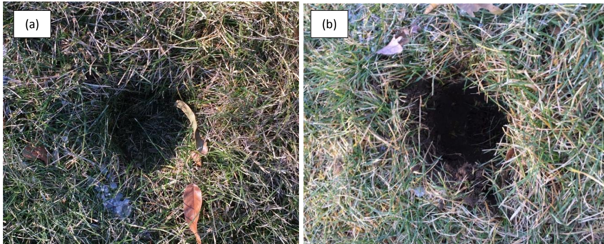
Figure 5-30: Impact craters of small spherical 7 kg weight (S1) dropped from (a) 15 m and (b) 30 m
