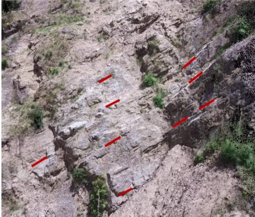
Figure 3-27: Illustration of foliation controlling failure and measurement location in 3D point cloud
