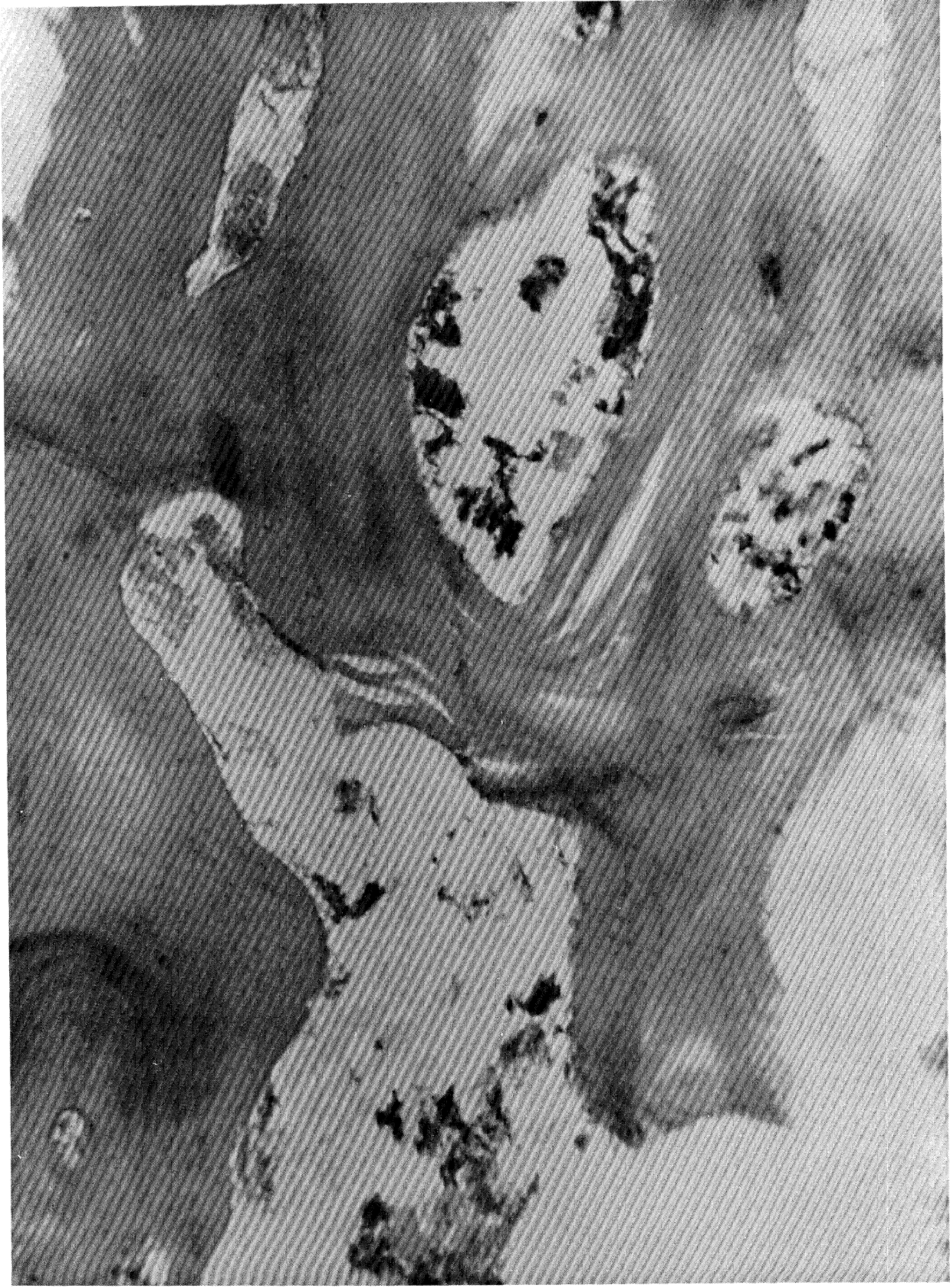
FIGURE 4. Micrograph of Failed Region of Diploë Layer
