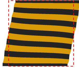
(b) \hat{\Sigma}_{21} = \Sigma applied on a 6 fiber volume element
