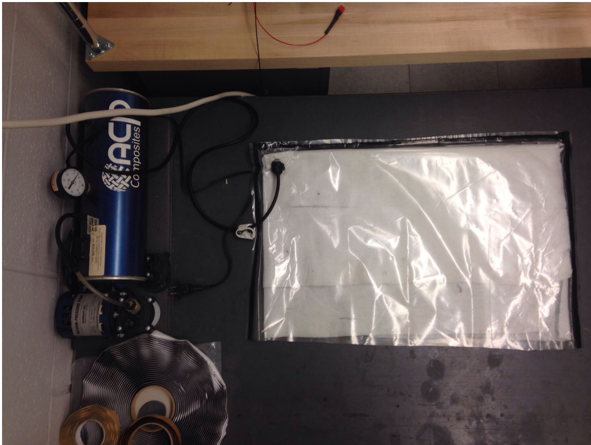
Figure 5.7: Experimental setup for vacuum bagging procedure
