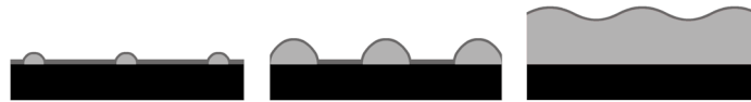
Figure 4.3. Schematic showing the modeled approximation of lithium deposits as a uniform square array of hemispheres that grow and eventually impinge during electrodeposition and that contract and separate during
