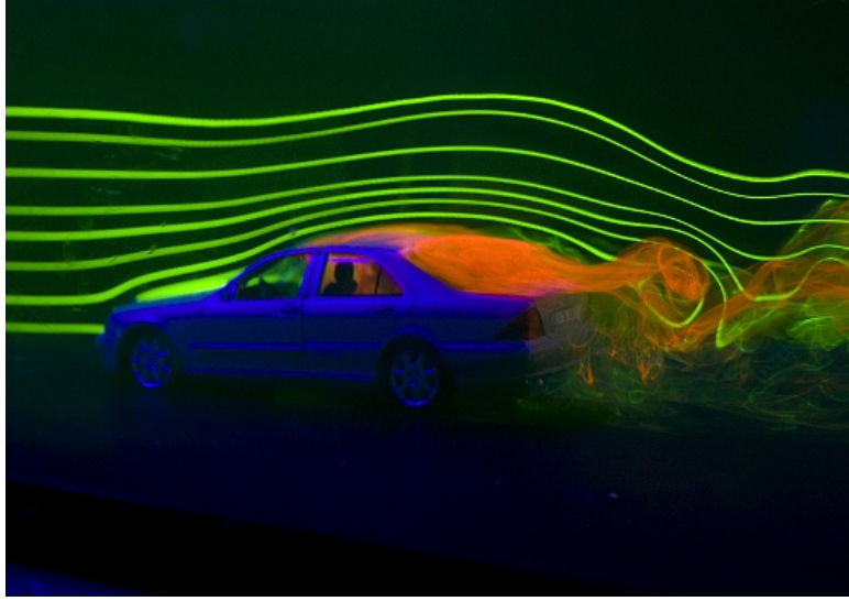
Figure 1.9: Visualization of air-flow separation of the rear end of an automobile. Photo credit: NASA [6].
