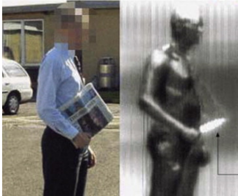
Figure 1.4 Terahertz image of men with a non-metallic knife hidden with a newspaper. [13]
