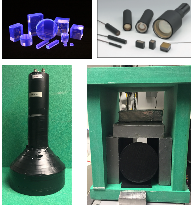
Figure 3.7 EJ-204 organic scintillator and photo-multiplier. To block room light, scintillator–PMT assembly was sealed with black tape. The assembly was surrounded by 5cm-thick lead bricks and borated plastics and only front side was opened and directed to the target allowing signals from an interaction to be recorded
