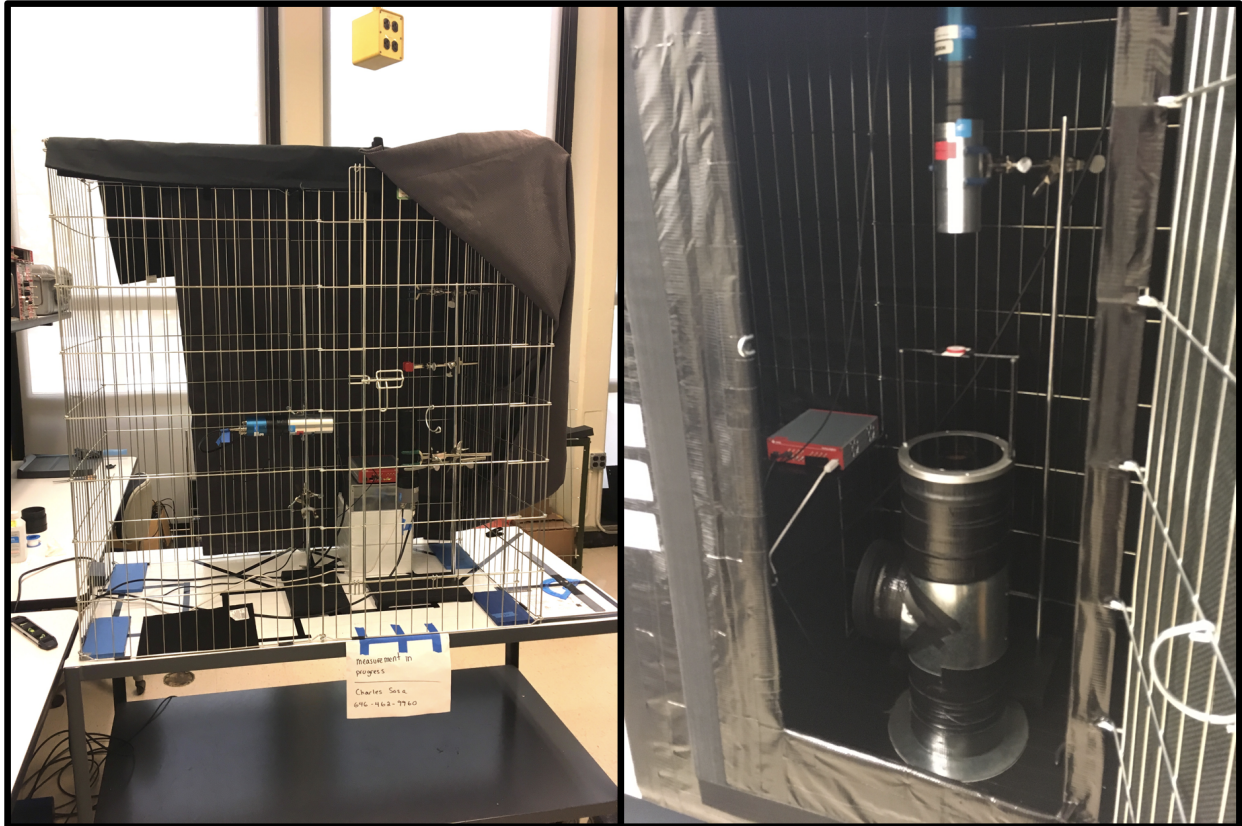
Figure 3.4: A light-tight compartment to support all experiments discussed in this work. The cage was large enough to accommodate all experiments and was necessary to avoid light leakage to certain PMTs that were large in diameter as compared to the tested scintillators.
