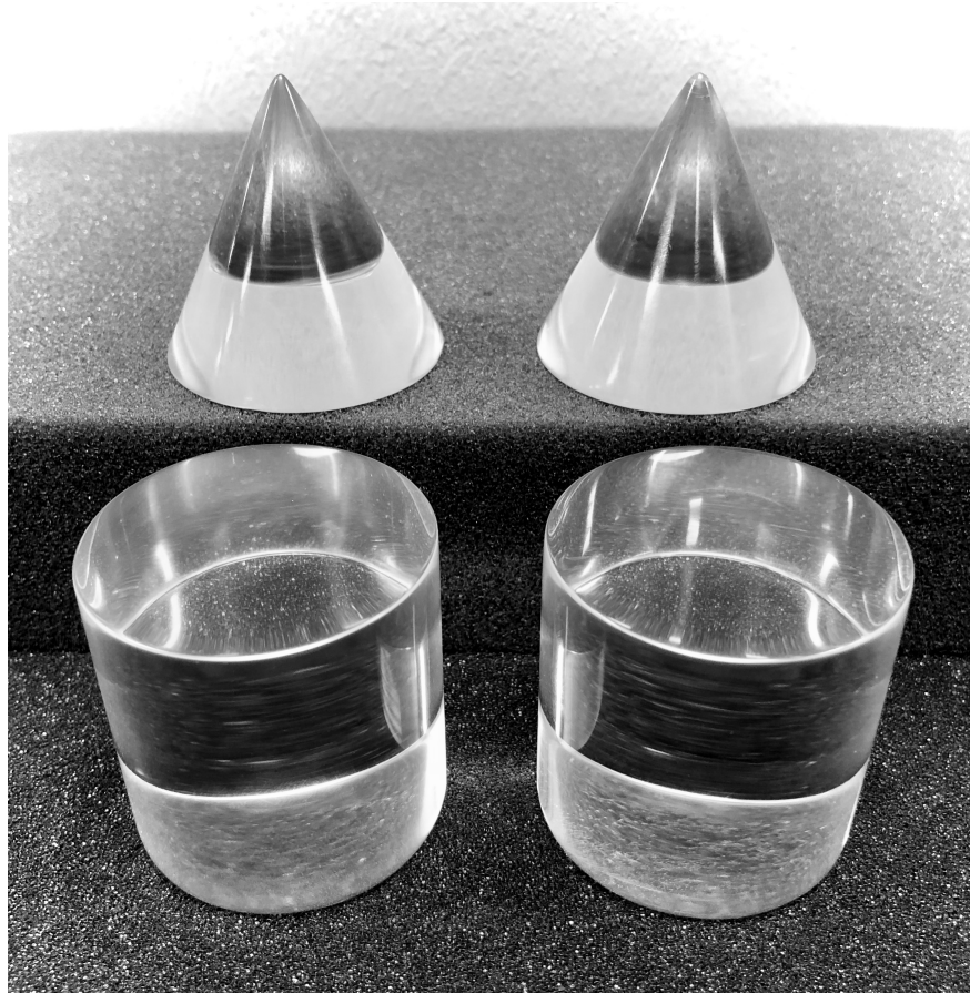
Figure 5.1: A picture of the four polished organic scintillators (EJ200) used in this chapter.
