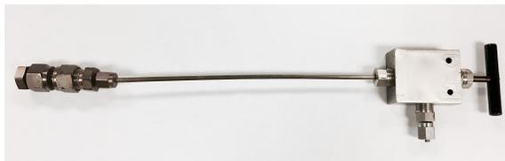
Figure 2.1: Photograph of a batch reactor with the gas valve attachment.
