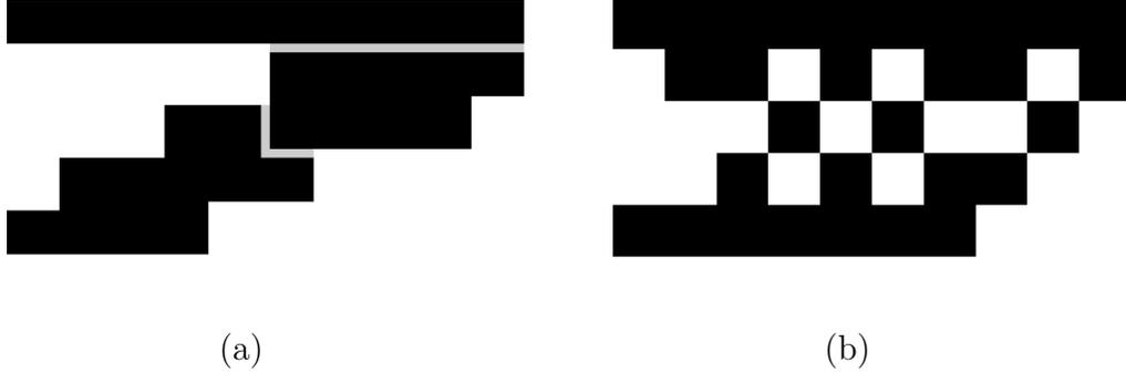
Figure 3.7: A comparison between the multi-component topology and conventional, single-piece topology for the cantilever example. (a) The optimized multi-component cantilever topology design. The gray regions indicate joint locations (assuming spot-welding joints) with the smaller Young’s modulus than base structural materials; (b) the conventional, single-piece cantilever topology design.
