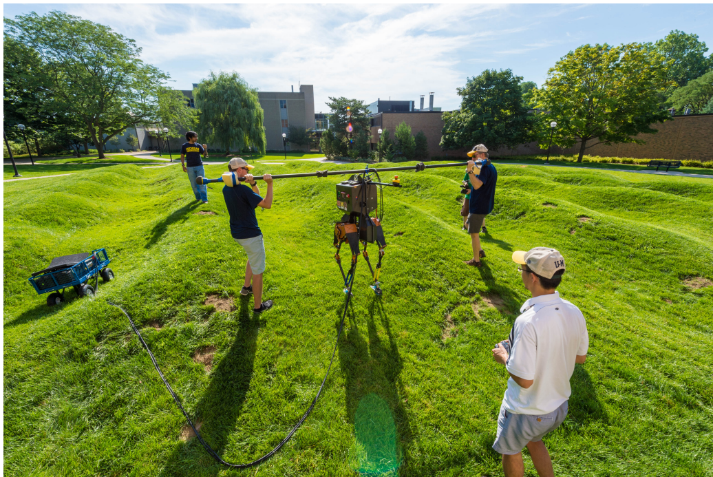
Figure 5.1: Bipedal robot MARLO walked on the University of Michigan’s Wave Field, a sinusoidally varying grass terrain. Photo was taken by Roger Hart.
