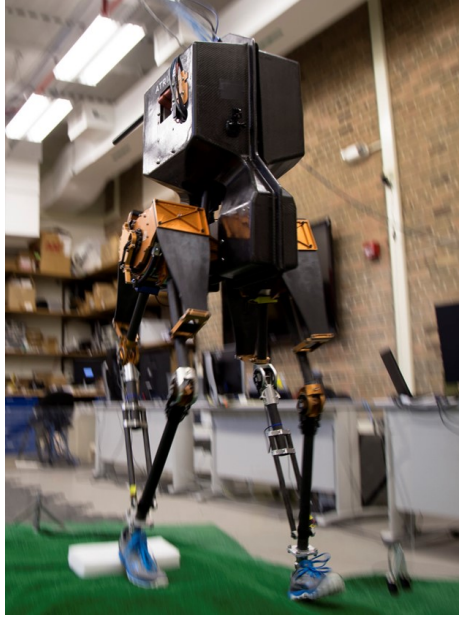
Figure 3.1: MARLO, an ATRIAS 2.1 bipedal robot. ATRIAS-series robots were designed by Jonathan Hurst and the Dynamic Robotics Laboratory at Oregon State University. (Photo: Evan Dougherty)
