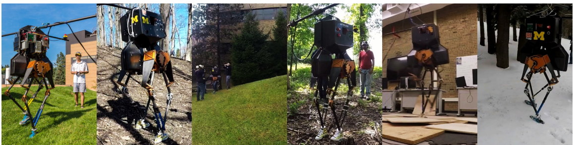
Figure 1.1: MARLO Experiment Summary. MARLO walking blind with passive feet. The feedback algorithms are tested on challenging terrain outdoors. While these images mostly show successes, sometimes the robot fails spectacularly, such as the robot catching fire while the Discovery Channel was filming. Failures, breaking the robot, and repairing it are all important learning experiences.
