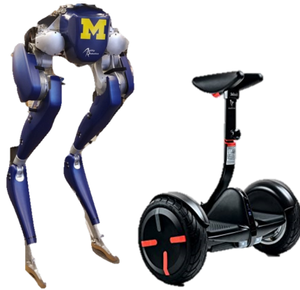
Figure 7.1: Cassie with a Segway. Cassie should drive the Segway miniPro as a human to move forward and backward, over flat ground and slopes, make turns and stop.
