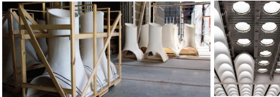
Figure 4.21. Dome-shaped coffers fabricated by Georgia-Pacific Gypsum LLC
