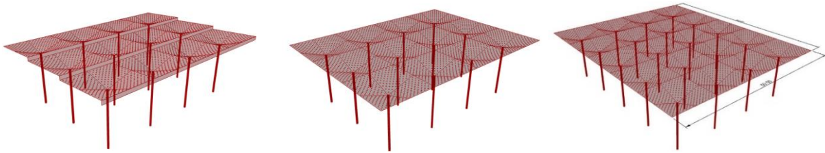
Figure 7.41. As-built High Life Textile Factory (a); eliminating North light (b); adjusting the size of each umbrella unit and arraying them in a 4 by 5 grid to cover a 50 by 60-m space (c)
