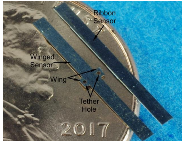
Fig. 3.12: Au-In bonded (a) winged sensor and (b) ribbon sensor coated with 1000 Å \text{Al}_2\text{O}_3 .
