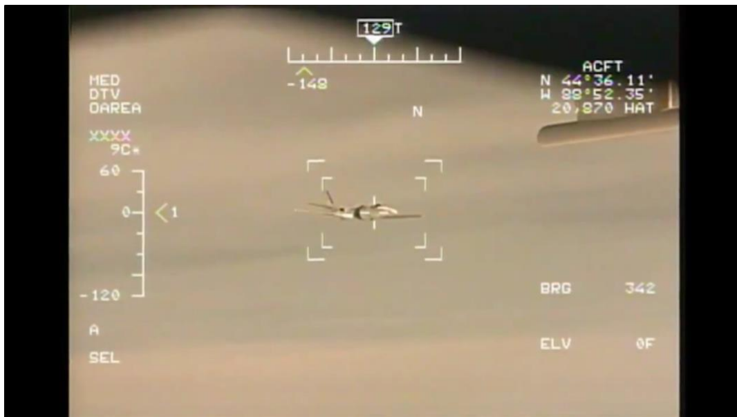
Figure 14. Predator B UAS operator/sensor screen showing targeting functions (source: DHS, CBP, Office of Public Affairs, Visual Communications Division, “CBP UAS B-Roll” (2012), Defense Video Imagery Distribution System , https://www.dvidshub.net/video/142871/cbp-uas-b-roll )
