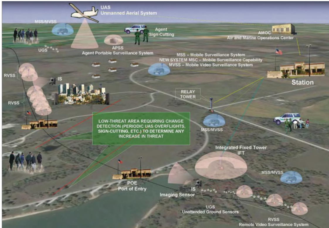
Figure 18. Elements of change detection capability (source: Department of Homeland Security (DHS), Customs and Border Protection, Office of the Border Patrol, 2012-2016 Border Patrol Strategic Plan (n.d.), 14)
