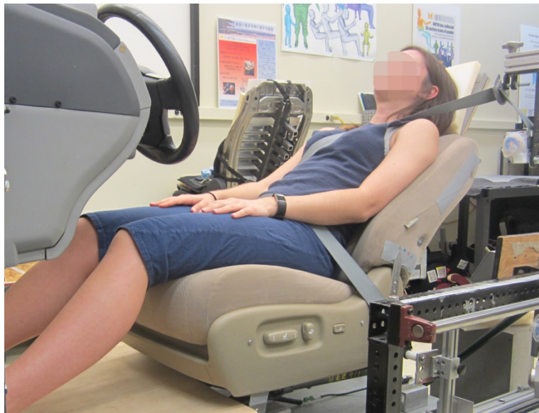
Figure 3. Test seat with power recline.
