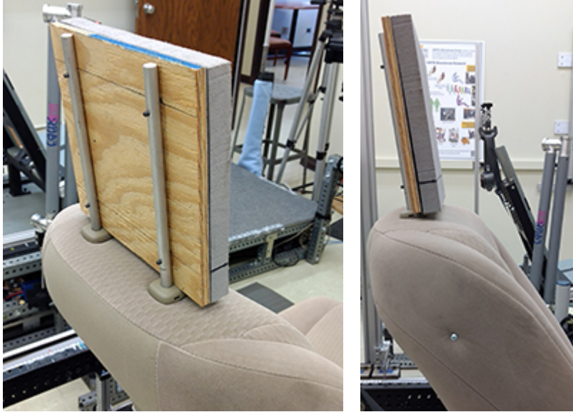
Figure 4. Removable head rest base. Additional padding was applied to obtain comfortable supported head positions – see text.
