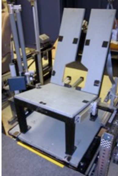
Figure 11. Hardseat with back opening (left) that allows access to posterior spine and pelvis as shown in center photo.
