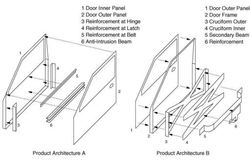
Fig. 9. Two automobile door structures with different product architectures.
