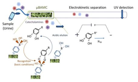
Figure 9. Schematic illustration of the different steps of cis-diols compounds analysis: preconcentration and purification on the integrated  $\mu$ BAMC unit, acidic elution, CZE separation and UV detection. Reprinted from [141] with permission.
