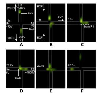
**Figure 13.** Multistacking by FASI-MSS in a T-shaped microfluidic chip. Evolution of the stacking zones depending on time (A–F). Rhodamine 6G was injected simultaneously from two streams (R1 and R3) prior to injection into the separation channel (R2 to R4). Reproduced from [171] with permission.
