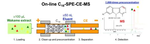
**Figure 10.** Schematic illustration of the online  $C_{18}$  SPE-CE-MS system. The  $C_{18}$  sorbent packed microcartridge was connected between the two pieces of separation capillary contained by two frits. Reprinted from [143] with permission. analytical systems and are potentially suitable for online coupling with CE analysis.
