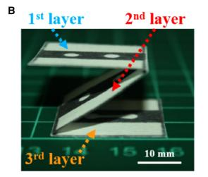
Figure 8. (A) Exploded view of  $\mu$ PAD structure and (B) Side view of folded  $\mu$ PAD layers. Reproduced from [127] with permission from Springer Nature.
