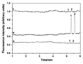
**Figure 12.** Electropherograms from the analysis of cefalexin (peak 1) and cefadroxil (peak 2) obtained by (A) FASS-sweeping and (B and C) REPSM-sweeping. The analyte concentration in (A, B) and (C) was 1400 ng/L and 60 ng/L, respectively. Reproduced from [160] with permission.
