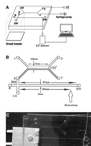
**Figure 11.** (A) Schematic diagram of the extract-CE glass chip; (B) top view of the chip, the grey part of channels is hydrophobic while the other parts are hydrophilic; (C) a photo of the extraction-CE microchip. Reproduced from [151] with permission.
