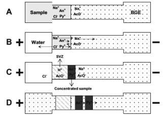
**Figure 2.** Schematic of the tITP-CZE method with a system induced terminator. (A) the capillary is filled with BGE and the sample is injected, (B) Na<sup>+</sup>, An<sup>+</sup>, and Py<sup>+</sup> migrates electrophoretically to the cathode and AcO<sup>-</sup> and Cl<sup>-</sup> to the anode electrophoresis, (C) a sample vacancy zone (SVZ) is formed and analytes are concentrated by tITP, and (D) separation of the analytes by CZE. Reproduced from [86] with permission.
