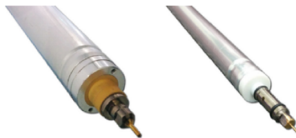
Figure 5: New small monitored drift tubes with a radius of 7.5 mm in comparison to normal monitored drift tubes with a radius of 30 mm. Both use the same gas mixture, wire voltage, and other internal parameters other than the tube radius.
